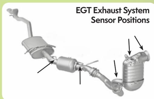
The above image indicates the multiple EGT sensor positions in an exhaust system. Some vehicles may have up to 6 EGT sensors fitted pre and post DPF / pre and post turbo charger / pre and post catalytic converter.
